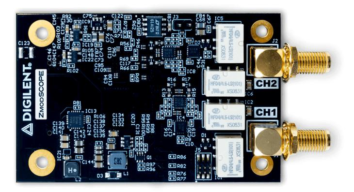
The Zmod Scope was designed to be a piece in a modular, HW and SW open-source ecosystem. The Zmod Scope can acquire two signals, with simultaneous sampling. Combined with a SYZYGY<sup>TM</sup> carrier, other SYZYGY<sup>TM</sup> compatible pods, Zmod Scope can be used for a variety of applications: data acquisition systems, closed loop controllers, scopes, etc.
