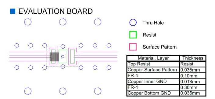
\* Line width should be designed to mach 50 ohm characteristic impedance depending on PCB material and thickness.
