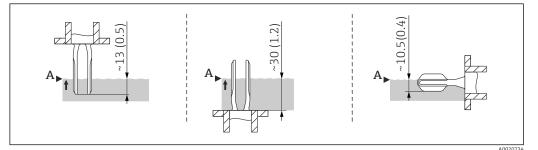
Orientation: vertical from above, vertical from below, horizontal; dimensions in mm (in)
