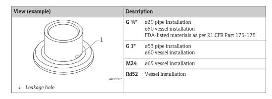
If installed horizontally and weld-in adapters with a leakage hole are used, ensure that the leakage hole is pointing down. This allows leaks to be detected as quickly as possible.
