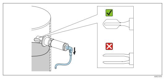
$\blacksquare 10$  Position of the fork in the case of horizontal installation in a vessel
