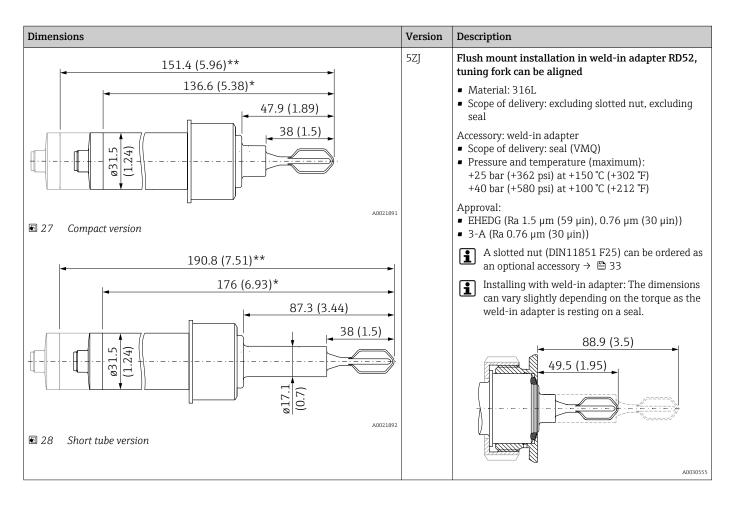
Pay attention to the temperature and pressure specifications for seals and clips used at the customer site.
