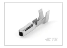
Terminal Type: Receptacle Mating Tab Width: 1 mm [.039 in ] Mating Tab Thickness: .64 mm [.025 in ] Terminal Transmits: 0 – 24 A (Low Power) Wire Size: 22 – 20 AWG
