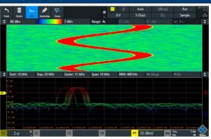
A spectrogram displays the spectrum of frequencies as they vary over time. For easy interpretation, the magnitude can be color-coded. Thanks to the high FFT rate, even fast frequency changes can be displayed.
