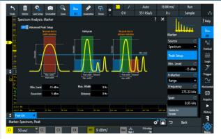
Markers can be automatically positioned on the frequency peaks for fast analysis. An adaptable threshold defines the peaks. Parameters such as excursion and maximum peak width can be adjusted for in-depth analysis. Results can be compiled in a table. Selectable delta measurements make it easy to adjust the distances between signal peaks.
