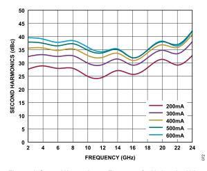
Figure 72. Second Harmonics vs. Frequency for Various  $I_{DQ}$  Values,  $V_{DD}$  = 15 V,  $P_{OUT}$  = 16 dBm
