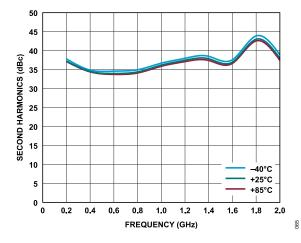
Figure 65. Low Frequency Second Harmonics vs. Frequency for Various Temperatures,  $V_{\rm DD}$  = 15 V,  $I_{\rm DQ}$  = 500 mA,  $P_{\rm OUT}$  = 16 dBm
