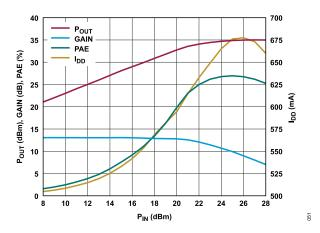
Figure 51.  $P_{OUT}$ , GAIN, PAE, and  $I_{DD}$  vs.  $P_{IN}$ , 4 GHz,  $V_{DD}$  = 15 V,  $I_{DQ}$  = 500 mA
