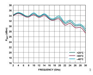
Figure 37.  $P_{SAT}$  vs. Frequency for Various Temperatures, 2 GHz to 28 GHz,  $V_{DD}$  = 15 V,  $I_{DQ}$  = 500 mA
