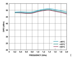
Figure 70. Low Frequency OIP2 vs. Frequency for Various Temperatures,  $V_{DD}$  = 15 V,  $I_{DQ}$  = 500 mA,  $P_{OUT}$  = 16 dBm
