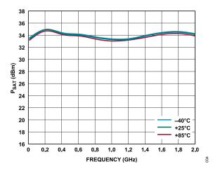
Figure 34.  $P_{SAT}$  vs. Frequency for Various Temperatures, 10 MHz to 2 GHz,  $V_{DD}$  = 15 V,  $I_{DQ}$  = 500 mA
