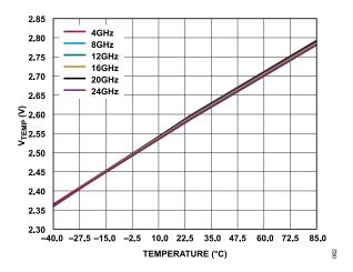
Figure 82.  $V_{TEMP}$  vs. Temperature for Various Frequencies,  $P_{OUT}$  = 28 dBm,  $V_{DD}$  = 15 V,  $I_{DQ}$  = 500 mA
