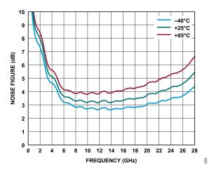
Figure 31. Noise Figure vs. Frequency for Various Temperatures,  $V_{DD}$  = 15 V,  $I_{DQ}$  = 500 mA
