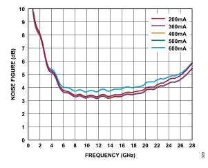
Figure 29. Noise Figure vs. Frequency for Various  $I_{DQ}$  Values,  $V_{DD}$  = 15 V
