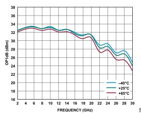
Figure 36. OP1dB vs. Frequency for Various Temperatures, 2 GHz to 28 GHz,  $V_{DD}$  = 15 V,  $I_{DQ}$  = 500 mA
