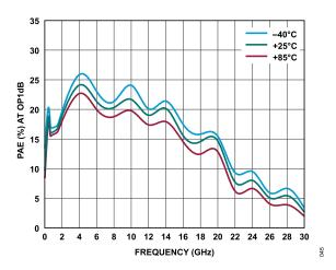
Figure 45. Power-Added Efficiency (PAE) at OP1dB vs. Frequency for Various Temperatures,  $V_{DD}$  = 15 V,  $I_{DO}$  = 500 mA
