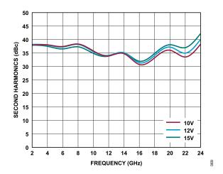
Figure 69. Second Harmonics vs. Frequency for Various  $V_{DD}$  Values,  $I_{DQ}$  = 500 mA,  $P_{OUT}$  = 16 dBm
