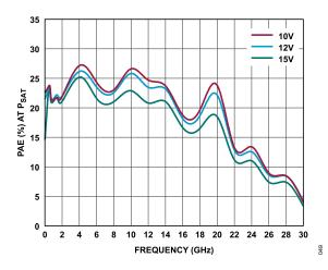
Figure 49. PAE at  $P_{SAT}$  vs. Frequency for Various  $V_{DD}$  Values,  $I_{DQ}$  = 500 mA
