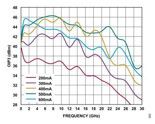
Figure 62. OIP3 vs. Frequency for Various  $I_{DQ}$  Values,  $P_{OUT}$  per Tone = 16 dBm,  $V_{DD}$  = 15 V
