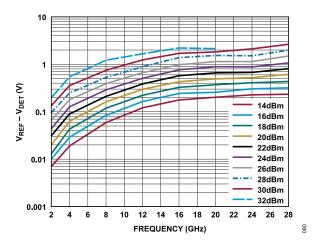
Figure 80. V<sub>REF</sub> - V<sub>DET</sub> vs. Frequency for Various P<sub>OUT</sub> Values
