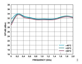
Figure 33. OP1dB vs. Frequency for Various Temperatures, 10 MHz to 2 GHz,  $V_{DD}$  = 15 V,  $I_{DQ}$  = 500 mA
