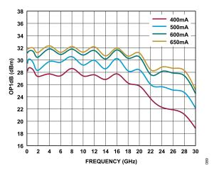
Figure 89. OP1dB vs. Frequency for Various Set-Point Drain Currents, Constant Current Mode, V<sub>DD</sub> = 15 V
