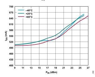
Figure 58.  $I_{DD}$  vs.  $P_{IN}$  for Various Temperatures, 16 GHz,  $V_{DD}$  = 15 V,  $I_{DQ}$  = 500 mA
