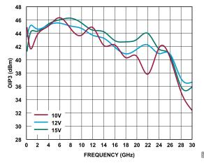
Figure 59. OIP3 vs. Frequency for Various  $V_{DD}$  Values,  $P_{OUT}$  per Tone = 16 dBm,  $I_{DQ}$  = 500 mA
