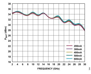
Figure 44.  $P_{SAT}$  vs. Frequency for Various  $I_{DQ}$  Values, 2 GHz to 28 GHz,  $V_{DD}$  = 15 V
