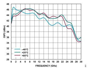
Figure 61. OIP3 vs. Frequency for Various Temperatures,  $P_{OUT}$  per Tone = 16 dBm,  $V_{DD}$  = 15 V,  $I_{DO}$  = 500 mA
