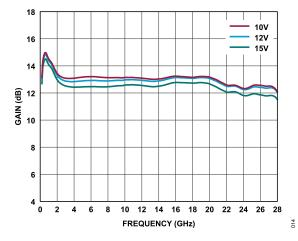
Figure 14. Gain vs. Frequency for Various  $V_{DD}$  Values, 200 MHz to 28 GHz,  $I_{DQ} = 500 \text{ mA}$
