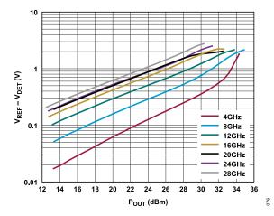
Figure 76. Detector Voltage (V<sub>REF</sub> - V<sub>DET</sub>) vs. P<sub>OUT</sub> for Various Frequencies
