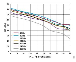
Figure 66. IM3 vs.  $P_{OUT}$  per Tone for Various Frequencies,  $V_{DD} = 15 \text{ V}$ ,  $I_{DQ} = 500 \text{ mA}$
