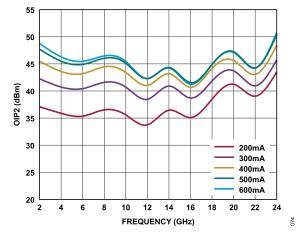
Figure 74. OIP2 vs. Frequency for Various  $I_{DQ}$  Values,  $V_{DD}$  = 15 V,  $P_{OUT}$  = 16 dBm
