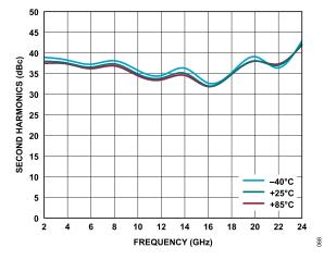
Figure 68. Second Harmonics vs. Frequency for Various Temperatures,  $V_{DD} = 15 \text{ V}$ ,  $I_{DQ} = 500 \text{ mA}$ ,  $P_{OUT} = 16 \text{ dBm}$
