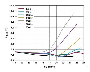
Figure 57.  $P_{DISS}$  vs.  $P_{IN}$  for Various Frequencies at  $T_A$  = 85°C,  $V_{DD}$  = 15 V,  $I_{DQ}$  = 500 mA
