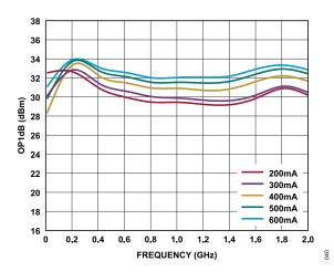
Figure 40. OP1dB vs. Frequency for Various  $I_{DQ}$  Values, 10 MHz to 2 GHz,  $V_{DD}$  = 15 V
