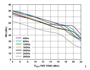
Figure 64. IM3 vs.  $P_{OUT}$  per Tone for Various Frequencies,  $V_{DD}$  = 12 V,  $I_{DQ}$  = 500 mA
