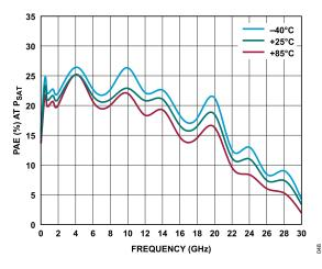
Figure 48. PAE at  $P_{SAT}$  vs. Frequency for Various Temperatures,  $V_{DD}$  = 15 V,  $I_{DQ}$  = 500 mA
