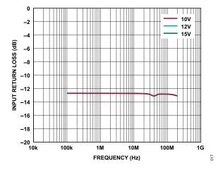
Figure 17. Input Return Loss vs. Frequency for Various  $V_{DD}$  Values, 100 kHz to 200 MHz,  $I_{DQ}$  = 500 mA
