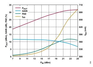
Figure 56.  $P_{OUT}$ , GAIN, PAE, and  $I_{DD}$  vs.  $P_{IN}$ , 24 GHz,  $V_{DD}$  = 15 V,  $I_{DQ}$  = 500 mA
