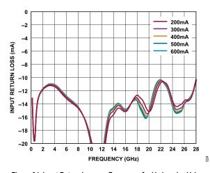
Figure 24. Input Return Loss vs. Frequency for Various  $I_{DQ}$  Values, 200 MHz to 28 GHz,  $V_{DD}$  = 15 V
