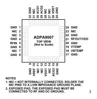
Figure 2. Pin Configuration
