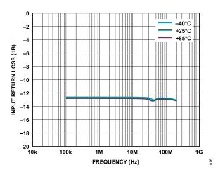
Figure 16. Input Return Loss vs. Frequency for Various Temperatures, 100 kHz to 200 MHz,  $V_{\rm DD}$  = 15 V,  $I_{\rm DQ}$  = 500 mA
