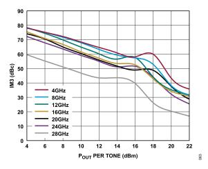
Figure 63. Third-Order Intermodulation Distortion (IM3) vs.  $P_{OUT}$  per Tone for Various Frequencies,  $V_{DD}$  = 10 V,  $I_{DQ}$  = 500 mA
