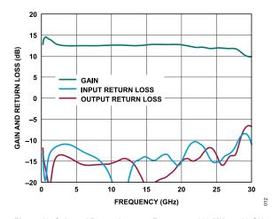
Figure 12. Gain and Return Loss vs. Frequency, 200 MHz to 30 GHz,  $V_{DD}$  = 15 V,  $I_{DQ}$  = 500 mA
