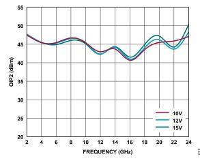
Figure 71. OIP2 vs. Frequency for Various  $V_{DD}$  Values,  $I_{DQ}$  = 500 mA,  $P_{OUT}$  = 16 dBm
