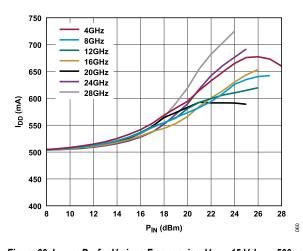
Figure 60.  $I_{DD}$  vs.  $P_{IN}$  for Various Frequencies,  $V_{DD}$  = 15 V,  $I_{DQ}$  = 500 mA
