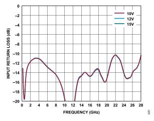
Figure 20. Input Return Loss vs. Frequency for Various  $V_{DD}$  Values, 200 MHz to 28 GHz,  $I_{DQ}$  = 500 mA
