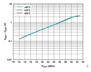
Figure 77. V<sub>REF</sub> - V<sub>DET</sub> vs. P<sub>OUT</sub> for Various Temperatures at 16 GHz
