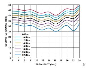
Figure 67. Second Harmonics vs. Frequency for Various  $P_{OUT}$  Values,  $V_{DD}$  = 15 V,  $I_{DQ}$  = 500 mA
