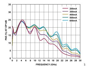
Figure 47. PAE at OP1dB vs. Frequency for Various  $I_{DQ}$  Values,  $V_{DD}$  = 15 V
