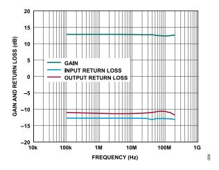
Figure 9. Gain and Return Loss vs. Frequency, 100 kHz to 200 MHz,  $V_{DD}$  = 15 V,  $I_{DQ}$  = 500 mA
