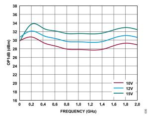
Figure 35. OP1dB vs. Frequency for Various  $V_{DD}$  Values, 10 MHz to 2 GHz,  $I_{DO}$  = 500 mA
