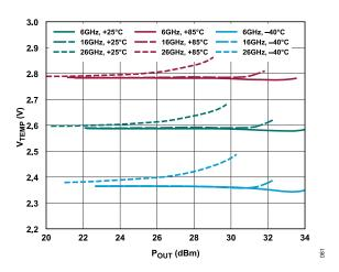
Figure 81. Temperature Sensor Voltage ( $V_{TEMP}$ ) vs.  $P_{OUT}$  for Various Frequencies and Temperatures,  $V_{DD}$  = 15 V,  $I_{DQ}$  = 500 mA
