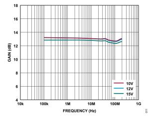
Figure 11. Gain vs. Frequency for Various  $V_{DD}$  Values, 100 kHz to 200 MHz,  $I_{DO}$  = 500 mA
