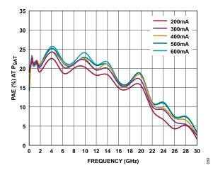
Figure 50. PAE at  $P_{SAT}$  vs. Frequency for Various  $I_{DQ}$  Values,  $V_{DD}$  = 15 V
