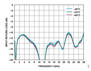
Figure 19. Input Return Loss vs. Frequency for Various Temperatures, 200 MHz to 28 GHz,  $V_{\rm DD}$  = 15 V,  $I_{\rm DQ}$  = 500 mA
