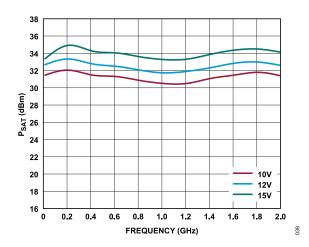
Figure 39.  $P_{SAT}$  vs. Frequency for Various  $V_{DD}$  Values, 10 MHz to 2 GHz,  $I_{DQ}$  = 500 mA
