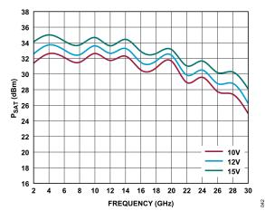
Figure 42.  $P_{SAT}$  vs. Frequency for Various  $V_{DD}$  Values, 2 GHz to 28 GHz,  $I_{DQ}$  = 500 mA
