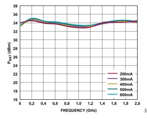
Figure 41.  $P_{SAT}$  vs. Frequency for Various  $I_{DQ}$  Values, 10 MHz to 2 GHz,  $V_{DD}$  = 15 V
