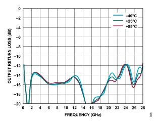
Figure 25. Output Return Loss vs. Frequency for Various Temperatures, 200 MHz to 28 GHz,  $V_{\rm DD}$  = 15 V,  $I_{\rm DQ}$  = 500 mA
