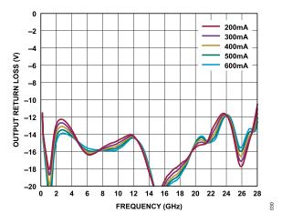
Figure 30. Output Return Loss vs. Frequency for Various  $I_{DQ}$  Values, 200 MHz to 28 GHz,  $V_{DD}$  = 15 V
