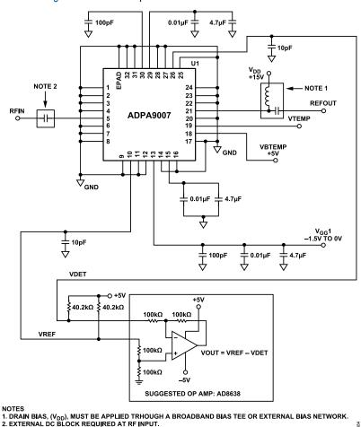
Figure 84. Basic Connections
