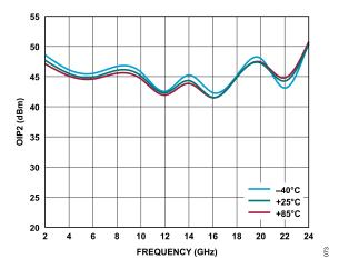
Figure 73. OIP2 vs. Frequency for Various Temperatures,  $V_{DD}$  = 15 V,  $I_{DQ}$  = 500 mA,  $P_{OUT}$  = 16 dBm
