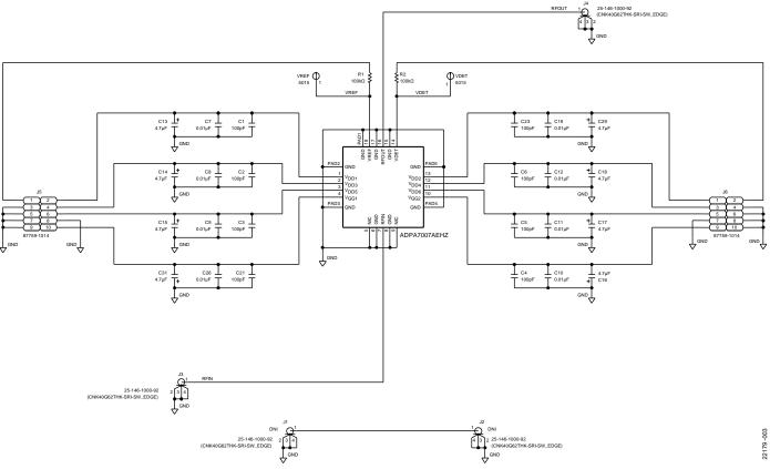
Figure 4. ADPA7007-EVALZ Evaluation Board Schematic
