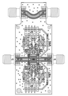
Figure 5. ADPA7007-EVALZ Assembly Drawing (Note That J1 and J2 Are Not Installed)
