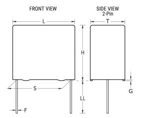
**General Information** Series PFR/F411 Dielectric Film/Foil Polypropylene Style Radial Features Pulse RoHS Yes Wire Leads Lead AEC-Q200 No Typical Component 0.625 g Weight An Operating Temperature Up To +105C Is Miscellaneous Allowed Under Certain Conditions. Please Consult KEMET For Details.
