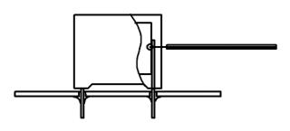
Temperature monitored inside the capacitor.
