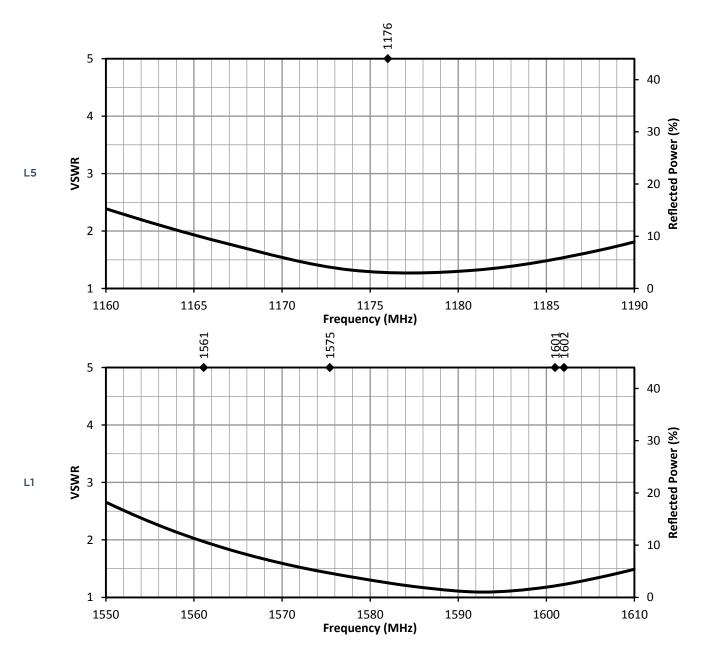
Figure 2. ANT-GNFPC-SHL15 Antenna VSWR with Frequency Band Highlights
