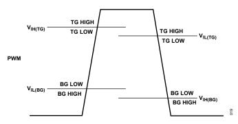
Figure 16. Three-State PWM Operation
