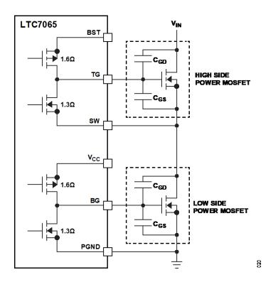
Figure 17. Simplified Output Stage in Half-Bridge Configuration
