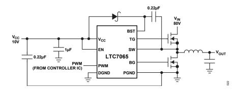
Figure 19. High Input Voltage Buck Converter
