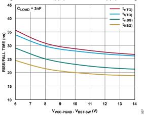
Figure 7. Rise and Fall Time vs. Driver Supply Voltage
