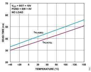
Figure 12. Dead-Time vs. Temperature
