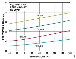
Figure 10. Propagation Delay vs. Temperature
