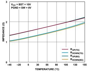
Figure 14.TG/BG Pull-Up and Pull-Down Resistance vs.
