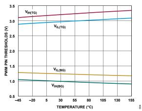
Figure 4. PWM Pin Thresholds vs. Temperature
