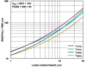
Figure 8. Rise and Fall Time vs. Load Capcitance
