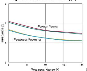
Figure 13. TG/BG Pull-Up and Pull-Down Resistance vs.
