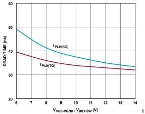
Figure 11. Dead-Time vs. Driver Supply
