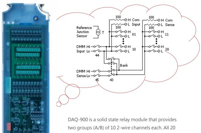
two groups (A/B) of 10 2-wire channels each. All 20 channels are switchable to high (HI) and low (LO) inputs, providing fully isolated inputs for the built-in digital meter or external instruments. During 4-wire resistance measurements, the channels of group A are automatically paired with the channels of group B to provide power and sense connections. The module has a built-in cold junction reference, which can greatly reduce errors caused by thermal gradients when measuring thermocouples
