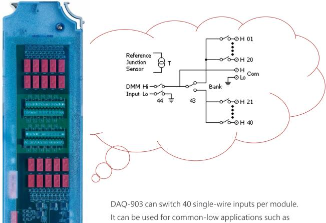
It can be used for common-low applications such as battery testing, component characterization and desktop testing. The low-voltage connection is isolated from ground and can be floated up to 300 V.
