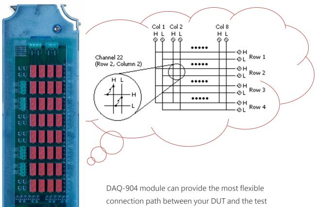
connection path between your DUT and the test system, allowing different test instruments to be connected to multiple points on the DUT at the same time.
