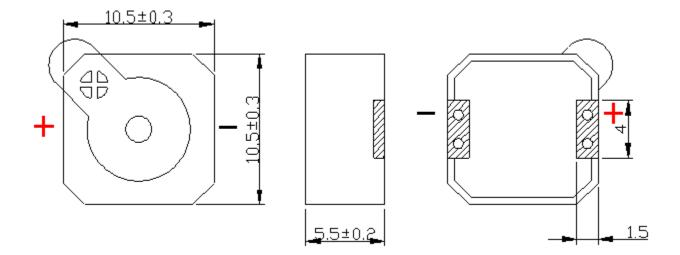
Attention: Must be installed with correct polarity.
