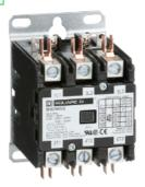
Contactor, Definite Purpose, 40A, 3 pole, 25 HP at 575 VAC, 3 phase, 24/24 VAC 50/60 Hz coil, with 2 mounting screws
