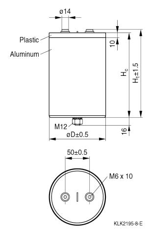
M12 stud on bottom of the aluminum case, nut (DIN 934) and toothed lock washer (DIN 6797) for fixing are standard for all types.
