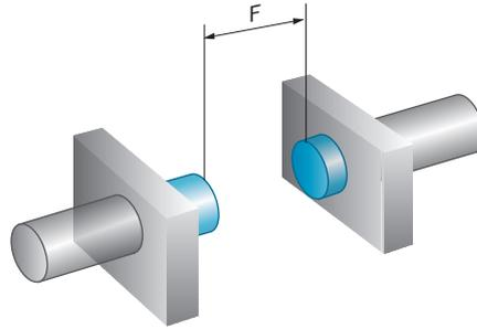
Mounting using BEF-KH-M0 bracket
