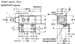
The L-shaped mounting bracket may also be attached to surface(A).
