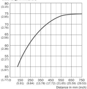
Minimum distance in mm (y) between the set sensing range (x) and white background (90 % remission)
