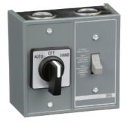
Manual Starter, fractional horsepower, duplex, 16A, 1 pole, 1 HP at 277 VAC, toggle and selector, no indicator, NEMA 1
