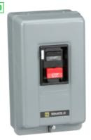
Manual Starter, integral horsepower, NEMA M1, 600 VAC, 2 pole, 3 HP at 230 VAC, single phase, no indicator, NEMA 1
