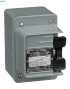
Manual Starter, fractional horsepower, 16A, 2 poles, 1 HP at 277 VAC, no indicator, NEMA 4 enclosure, 1 conduit opening
