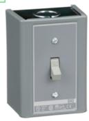
Switch, manual, 30A, 3 pole, 10 HP at 575 VAC, three phase, toggle operated, no indicator, NEMA 1 jumbo enclosure
