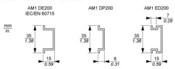
NOTE: Only size 1 (smallest) blocks can be installed on DIN rail with the TM7ACMP mounting plate.
