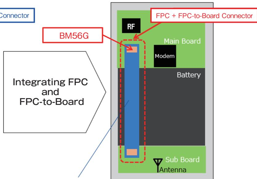
FPC can be placed on top of the battery
