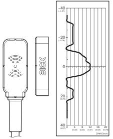
Assured switch on distance Sao 9 mm. Observe border areas for parallel approach: a minimum distance of 4 mm (typical) must be upheld when the actuator moves laterally to the sensor surface. This prevents early triggering due to the side preparation areas. "Flat"/"Mini" actuator, active front sensor surface
