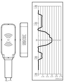
Assured switch on distance Sao 9 mm. Observe border areas for parallel approach: a minimum distance of 4 mm (typical) must be upheld when the actuator moves laterally to the sensor surface. This prevents early triggering due to the side preparation areas. "Flat"/"Mini" actuator, active front sensor surface
