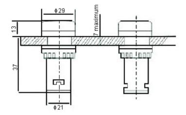
This superb range of LED lamps offers high illumination output, long life, low temperature and is supplied as a complete unit with encapsulated LED ready to fit. The range provides even lighting in each colour and is available in: White, amber, red, green and blue. 24V ac and DC. 110V ac (50Hz). 230V ac (50Hz).
