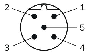
Connector M12, 5-pin, A-coded
