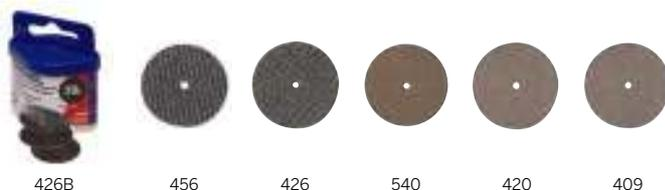
For slicing and cutting in metal, wood and plastic. Cut-off wheels make it easy to cut or slot bolts, screws, sheet metal, thin wood and plastic. Fiberglass reinforced cut-off wheels (456, 426, 426B) are for tough applications. The cut-off wheel cuts only along its edge. Do not attempt to sand or cut curved holes with cut-off wheels. Use Dremel cut-off wheels with mandrel 402.
