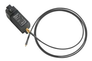
The TPR1000 and TPR4000 probes provide a low noise, large offset range solution for measurement of ripple on DC power rails ranging from -60 to +60 VDC. Tektronix's power rail probes offer industry leading low noise and high offset range required to measure AC ripple between 200  $\mu V_{p-p}$  and 800 mV<sub>p-p</sub> at up to 4 GHz.
