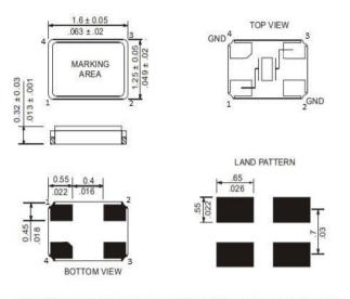
**Note:** According to ceramic base availability the Chamfer location could be on a different pin. However, the Chamfer's location does not influence the electrical performance of the crystal.
