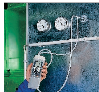
Simultaneous measurement of pressure and velocity flow using a Pitot tube
