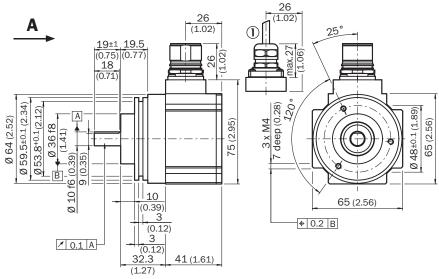
General tolerances according to ISO 2768-mk ① R = min. bending radius 40 mm
