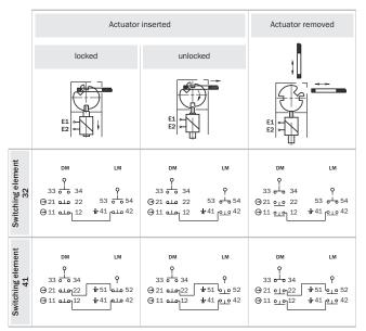
${}_{\ensuremath{\mathbf{W}}}$  Positive action N/C locking monitoring contact
