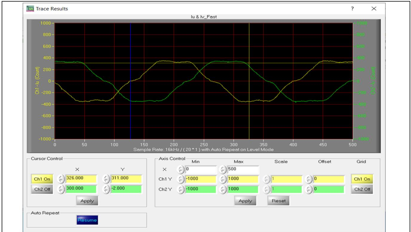
**Figure 9 Trace waveform for I<sub>u</sub> & I<sub>v</sub> open loop diagnostic**
