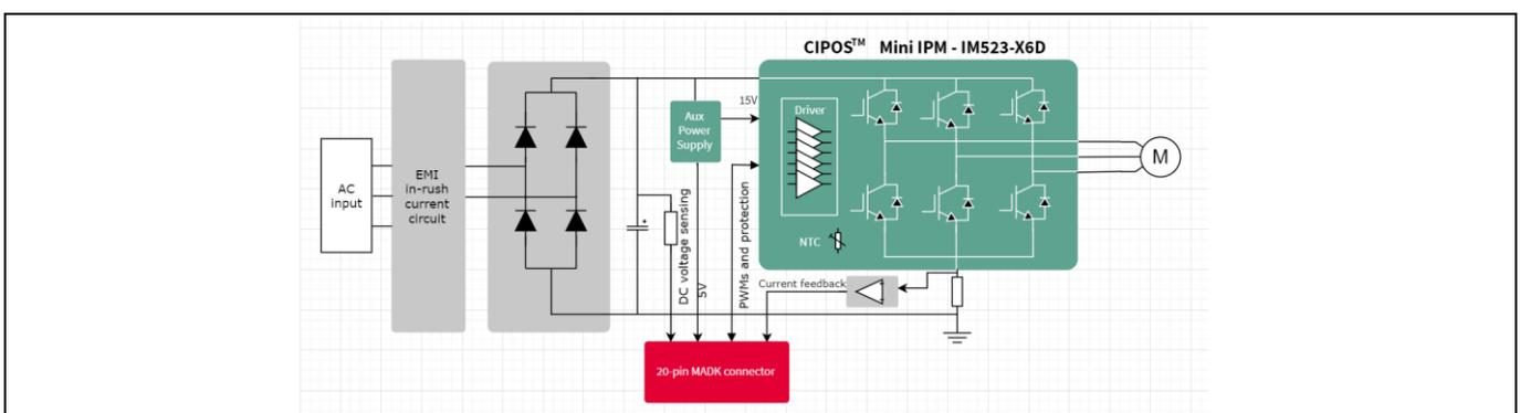
**Figure 2 Block diagram of the EVAL-M1-IM523 evaluation board**
