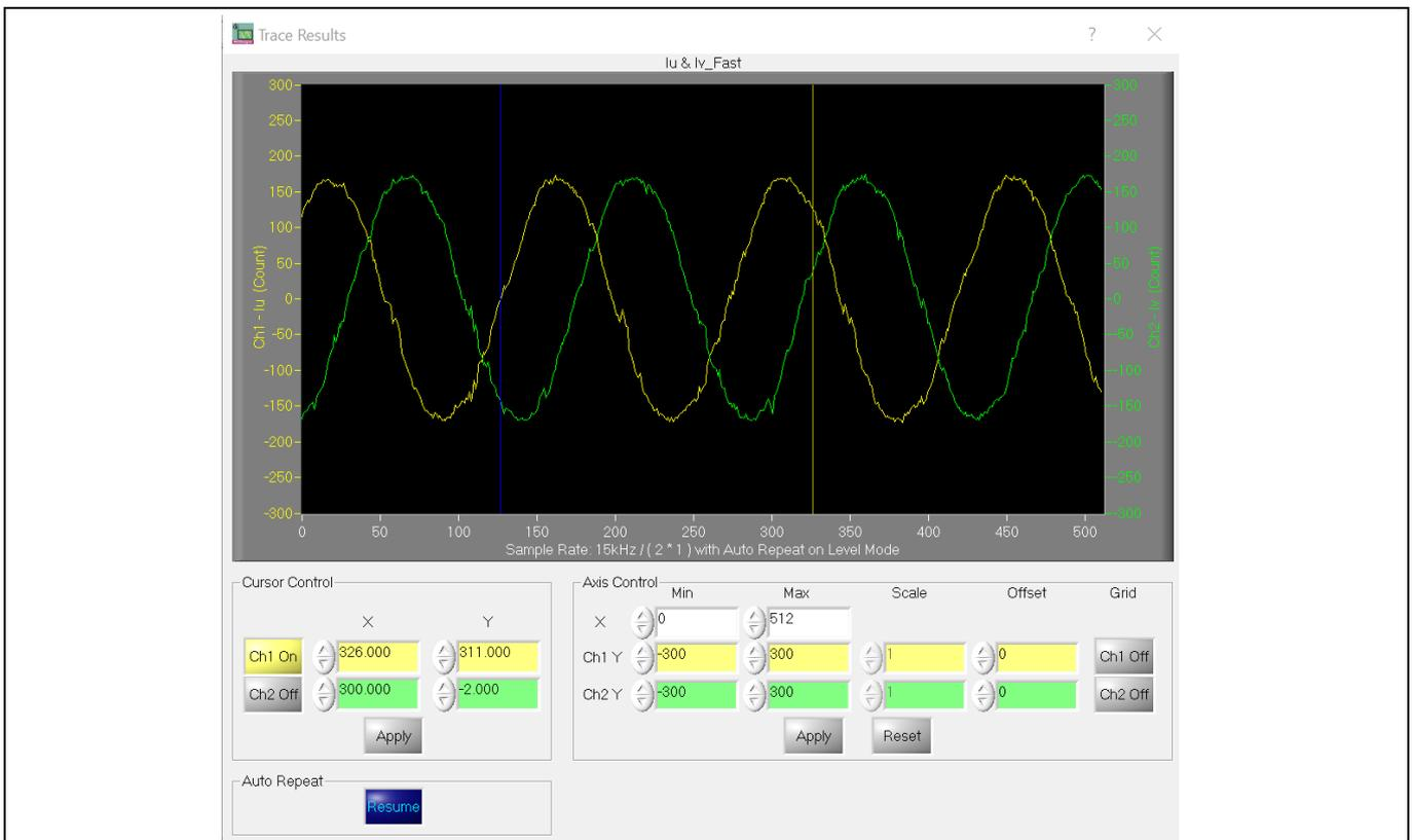
**Figure 38 930 W load, 5.5 A<sub>rms</sub> phase current, 15 kHz PWM, 220 V<sub>AC</sub> input**
