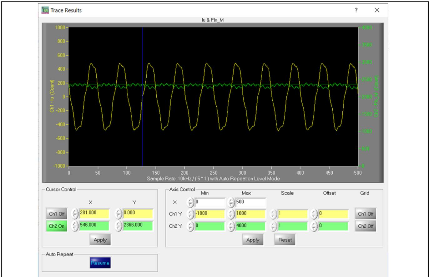
**Figure 10 Trace waveform for  $I_u$  &  $Flx-M$  at 50% speed**
