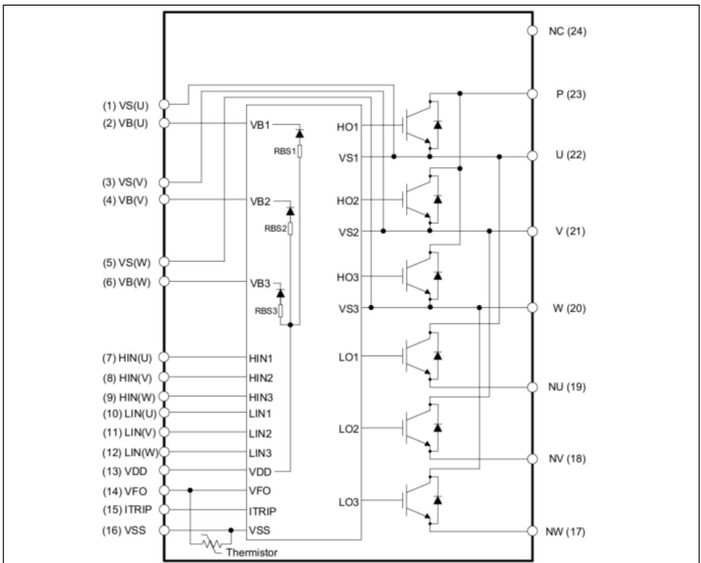
Figure 11 Internal block of the IM523-X6A
