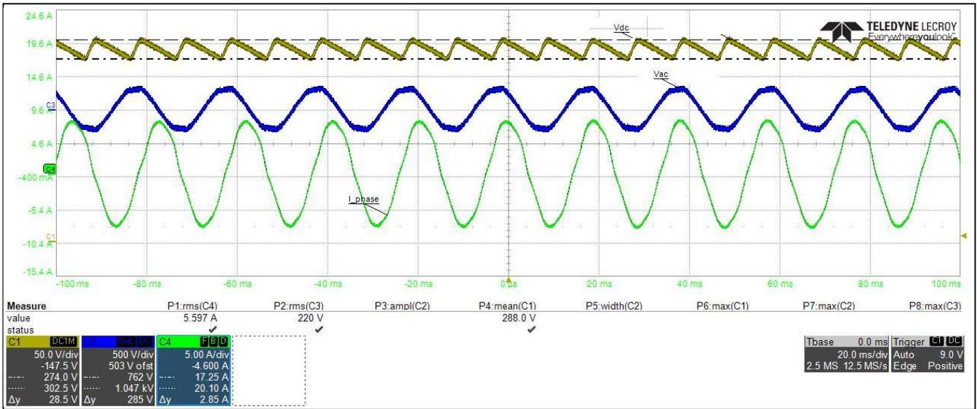
**Figure 28 Scope waveform at 220 V<sub>AC</sub> input, 15 kHz PWM and 900 W output**
