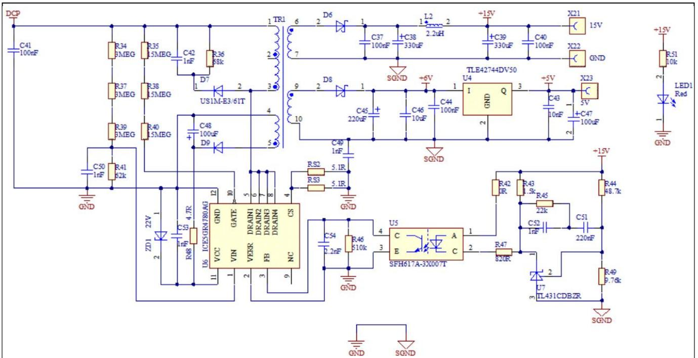
**Figure 14 Auxiliary power supply of the EVAL-M1-IM523**
