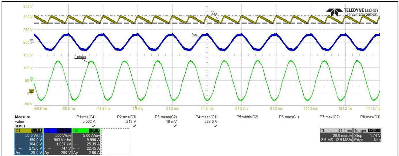
**Figure 39 Scope waveforms at 930 W load, 5.5 A<sub>rms</sub> phase current, 15 kHz PWM, 220 V<sub>AC</sub> input**
