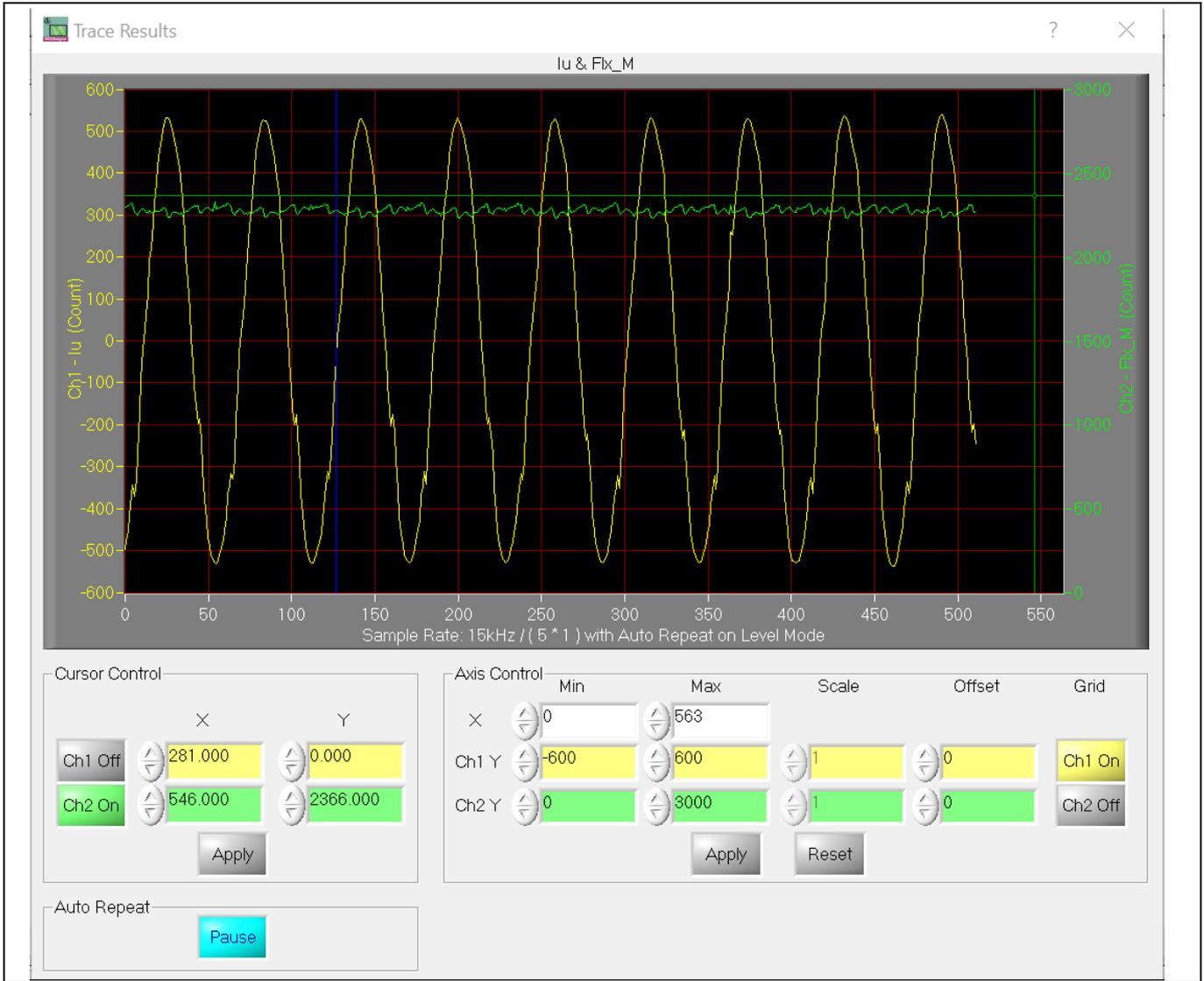
**Figure 26** iu & Flx\_M at 15 kHz PWM, 220 V<sub>AC</sub> input, 900 W output (5.5 A<sub>rms</sub> phase current)
