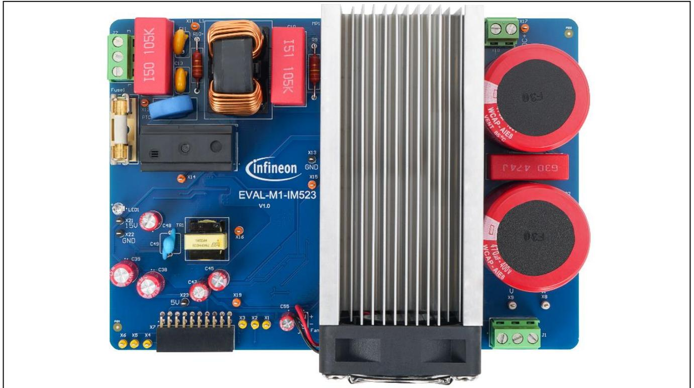
**Figure 15 Top-assembly PCBA of the EVAL-M1-IM523**
