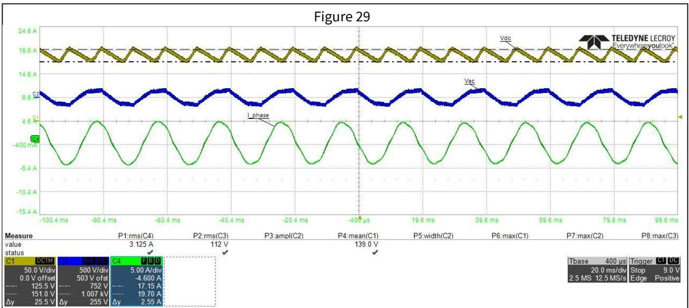
**Figure 29 Scope waveform at 110 V<sub>AC</sub> input, 500 W output power, and 15 kHz PWM**
