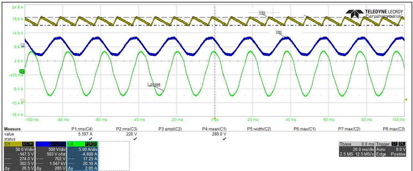
**Figure 22** 220 V<sub>AC</sub> input, V<sub>DC</sub> bus voltage ripple
