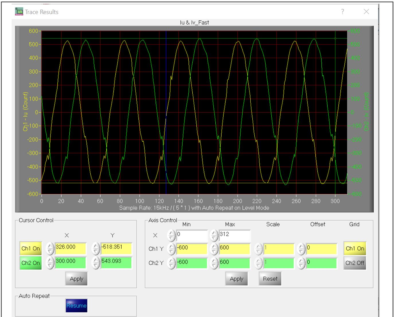
**Figure 25 Iu & Flx\_M at 15 kHz PWM, 220 V<sub>AC</sub> input, 900 W output (5.5 A<sub>rms</sub> phase current)**
