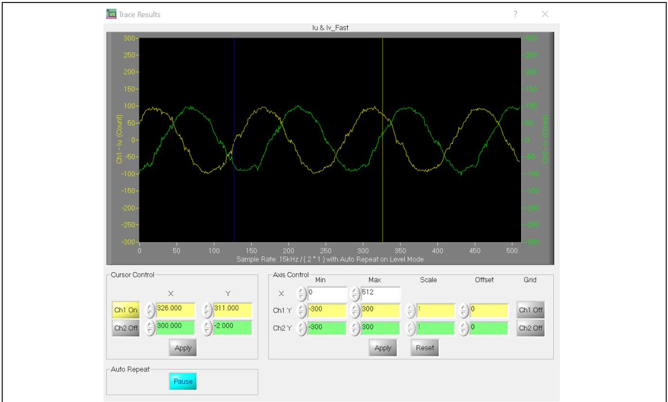
**Figure 37 500 W load current feedback, 3 A<sub>rms</sub> phase current, 15 kHz PWM, 220 V<sub>AC</sub> input**
