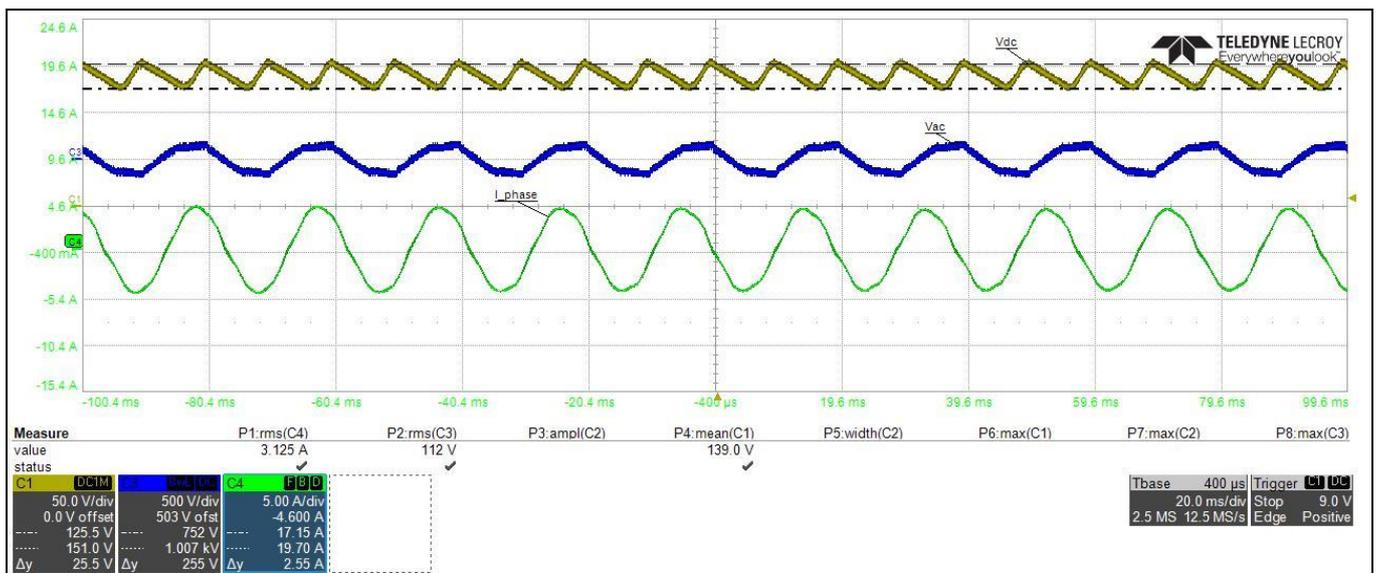
**Figure 23** 110 V<sub>AC</sub> input, V<sub>DC</sub> bus voltage ripple
