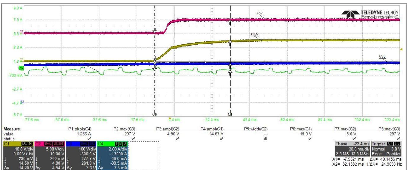
Figure 17 Power supply voltage (15 V & 5 V)
