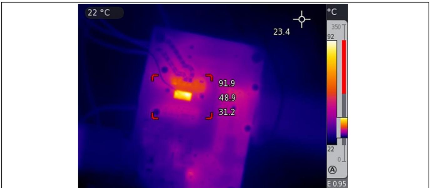
**Figure 27** Thermal test at 220 V<sub>AC</sub> input, 15 kHz PWM and 900 W output
