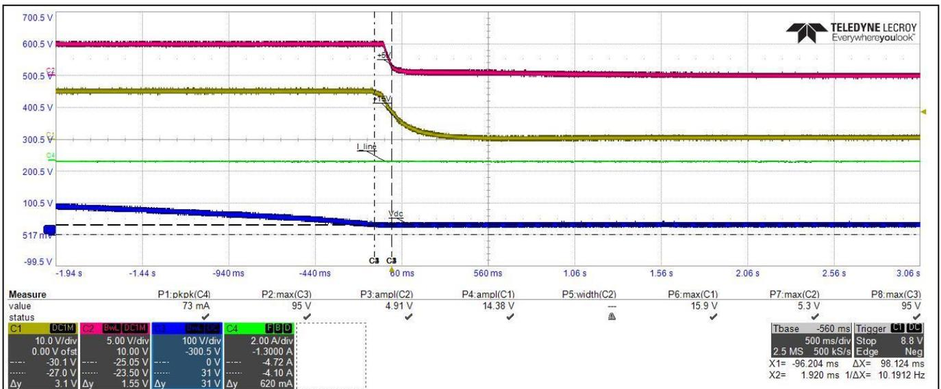
Figure 19 Input 85 V<sub>AC</sub>
