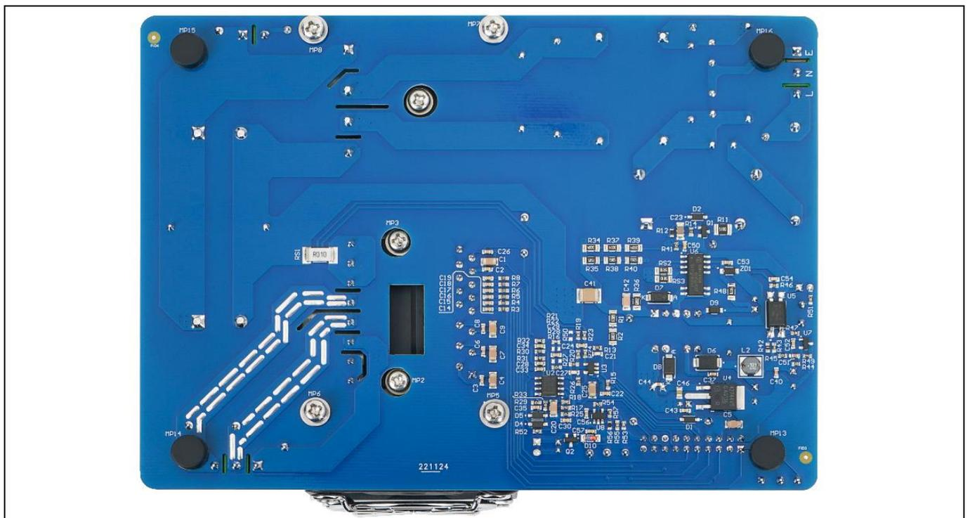
**Figure 16 Bottom-assembly PCBA of the EVAL-M1-IM523**
