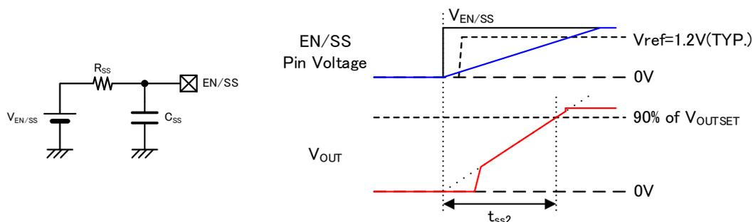
\* Definition of soft-start time : Time from  $V_{EN/SS}$  start-up until output voltage reaches 90% of set output voltage.
