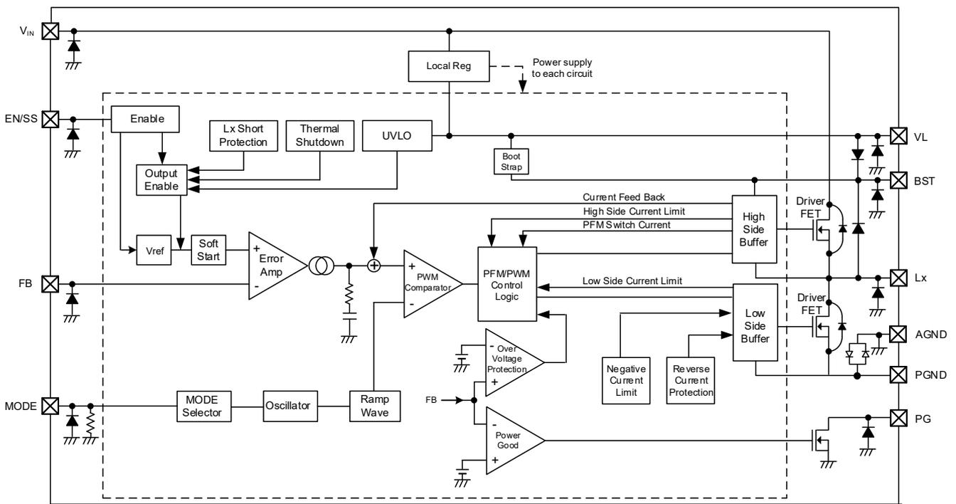
\* Diodes inside the circuit are ESD protection diodes and parasitic diode.
