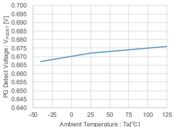
(20) PG Output Voltage vs. Ambient Temperature
