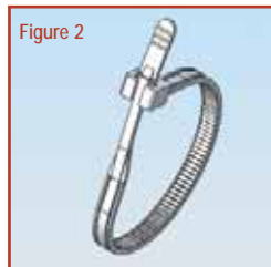
Figure 2 At Pre-lock Position
