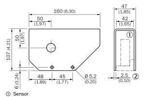
O Base plate with mounting material in scope of delivery
