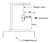
1 Meter From Microphone To Fan Intake
