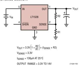
Figure 2. Adjustable Operation
