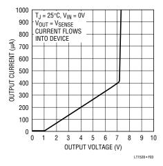
Figure 3. Reverse Output Current
