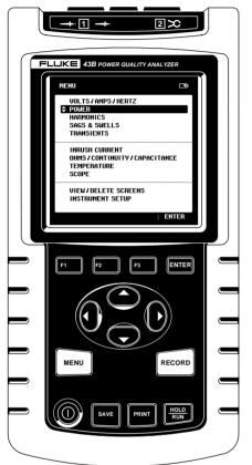
The Fluke 43 Power Quality Analyzer performs the measurements you need to maintain power systems, troubleshoot power problems and diagnose equipment failures. It combines a power quality analyzer, 20 MHz oscilloscope, a multimeter and a recorder in a single tool.
