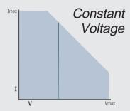
Constant voltage mode is used for load testing of constant current power supplies. The unit operates as a high power shunt regulator.
