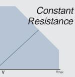
Constant resistance mode simulates a standard resistive load by providing a current drain proportional to voltage. Settings are displayed in Ohms or milli-Ohms.
