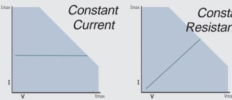
Constant current mode is used for load testing of normal voltage-source power supplies and for constant current discharge testing of batteries.
