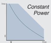
Constant power mode simulates a load whose power consumption is independant of the applied voltage. This is true of many types of equipment that incoporate switchmode regulators.
