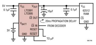
Figure 6. A Typical Nonvolatile CMOS RAM Application
