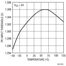
Reset Voltage Threshold vs Temperature
