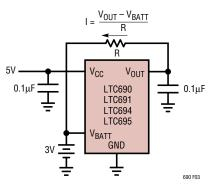
Figure 3. Charging External Battery Through  $V_{\mbox{OUT}}$
