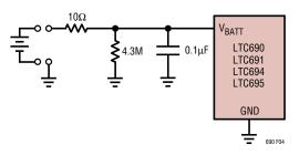
Figure 4. 10 $\Omega/0.1\mu F$  Combination Eliminates Inductive Overshoot and Prevents Spurious Resets During Battery Replacement
