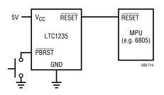
Figure 14. The External Push-Button Reset with the LTC1235
