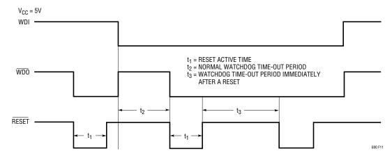
Figure 11. Watchdog Time-Out Period and Reset Active Time
