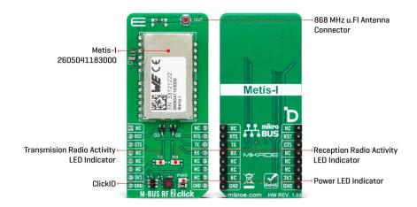
Communication between the Metis-I and the host MCU is made through a UART interface, using the standard UART RX and TX pins and hardware flow control pins (CTS/RTS). The module communicates at 115200bps by default, allowing efficient data exchange. The board also includes a reset (RST) pin for resetting the module. There are two LED indicators for user interaction: an orange TX LED signaling transmission activity and a yellow RX LED indicating reception.
