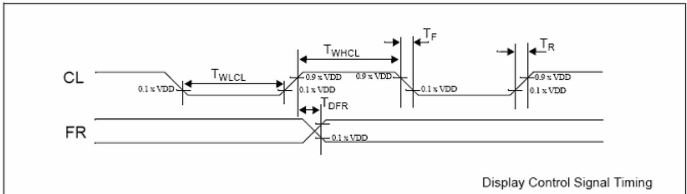
CL and FR timing characteristics at VDD=5 volts
