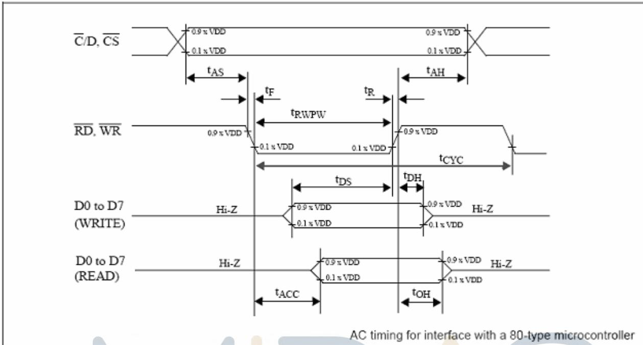
AC timing for interface with a 80-type microcontorller at VDD=5 volts VDD = 5 V ±10%; VSS = 0 V; Tamb = -20 °C to +75°C.
