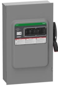
Safety switch, heavy duty, unfused, viewing window, NEMA 3R, 600V, 200A, 3 pole, neutral installed
