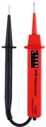
Meterman's VT500 is a two-pole tester that uses six LEDs to indicate voltages from 12 V to 400 V, either ac or dc. No battery is required; it is powered from the unit under test. The VT500 is an inexpensive way to measure voltage presence either ac or dc and display amplitude thresholds. This product is UL listed.
