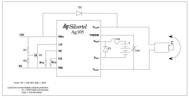
Figure 4: Typical System Diagram
