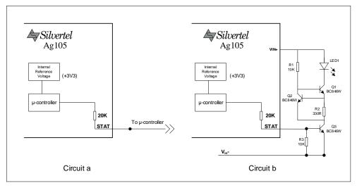
Figure 6: Status Pin output Configurations
