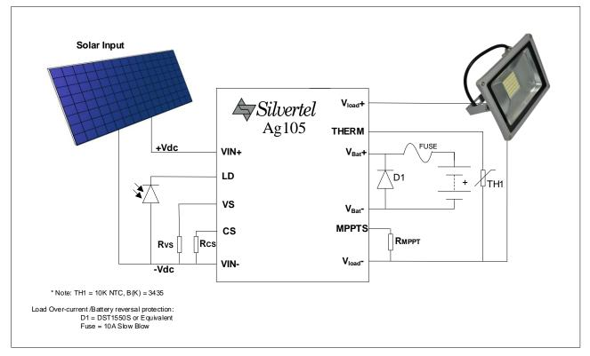
Figure 9: Solar Powered Light
