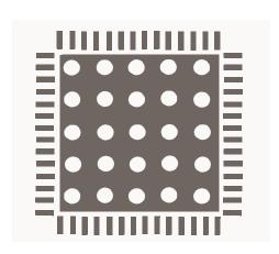
Figure 16-2a. Plot of the Solder Mask (White Area)
