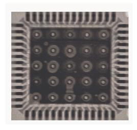
Figure 16-2b. X-Ray Image of the Assembly
