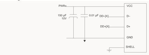
Figure 11-1. USB Downstream Port Connection
