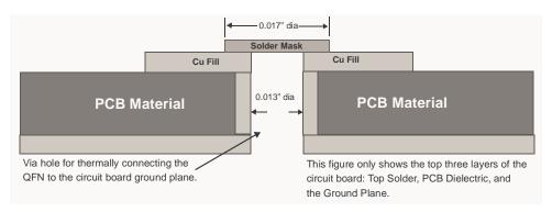
Figure 16-1. Cross-section of the Area Underneath the QFN Package
