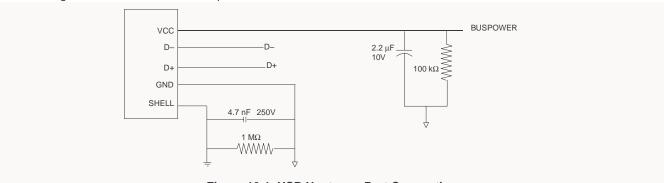
Figure 10-1. USB Upstream Port Connection
