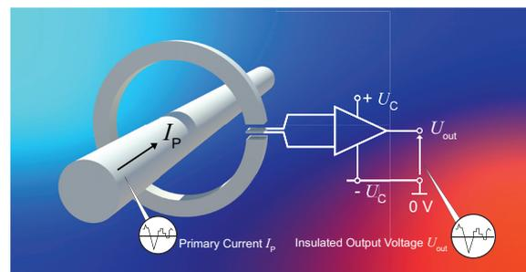
Fig. 1: Principle of the open loop transducer.
